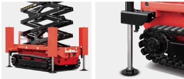
Equipped with one key outrigger leveling function, automatically adjust the frame to the level state, hydraulic outrigger to enhance the stability of the equipment. At the same time, it can also operate a single outrigger to meet the operation requirements under special working conditions.
